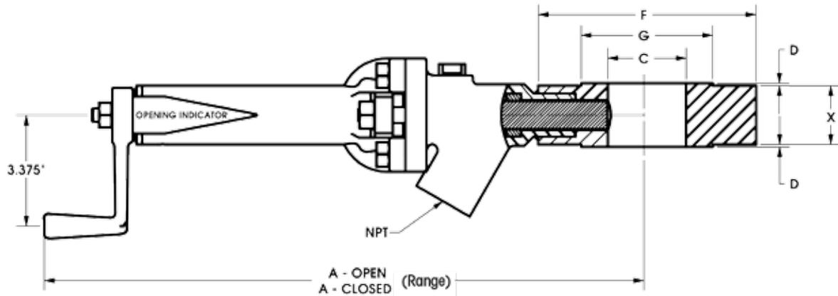
For use with Ram-Type Drain Valves a recess is required. Use piloting dimensions as discussed on page 10.
