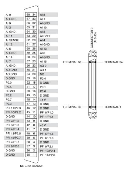
PCI/PXI-6221 (68-Pin) Pinout
