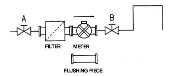
Figure 6 Flowmeter system without bypass
