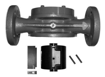
9. Install the vanes. Make sure the magnets are on the same side where the pulse transmitter is. If the flow meter has two magnets, install the vanes with the magnets on opposite side of each other.
