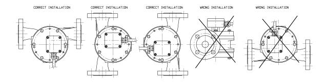
Figure 3 Installation flowmeter
