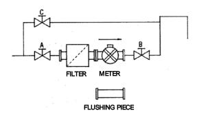
Figure 5 Flowmeter system with bypass
