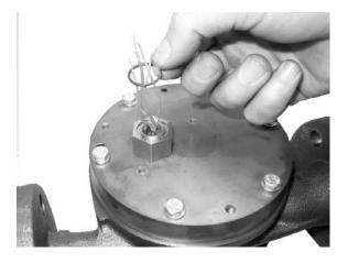
Remove the two spacers and the O-ring that is on the top of the pulse transmitter assembly.
