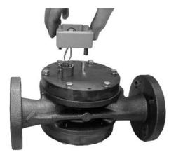
Remove the two crews in the mounting holes of the box, and remove the box. Two spacers will remain attached to the flow meter.
