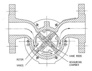
Figure 1 Sectional view of VAF vane meter
