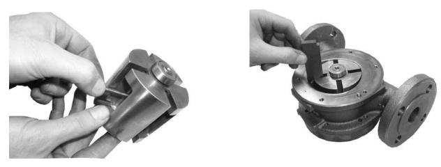
Clean rotor vanes and push rods with diesel oil.
