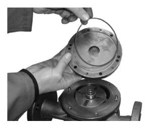
3. Lift the cover and remove the bolts and the O-ring.
