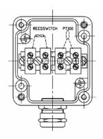
Figure 4 Electrical connection of pulse transmitter.
