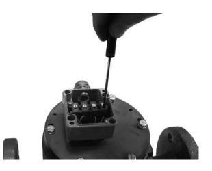
Disconnect the wiring (external and internal connections), pulse - red, temperature - green. Please make sure to write down how the connections are made.
