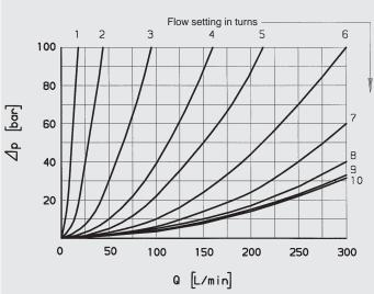
DRV Flow direction from B to A Pressure differential  $\Delta p$  depending on flow rate Q via opened check valve at  $v = 72 \text{ mm}^2/\text{s}$  and  $t_{oil} = 30 \text{ }^\circ\text{C}$
