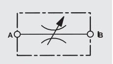
Flow control valves with reverse flow check DRV
