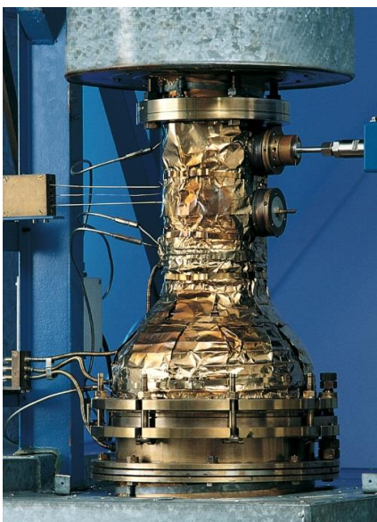
High temperature flow test bench HTP in closed construction „Universität Stuttgart“
